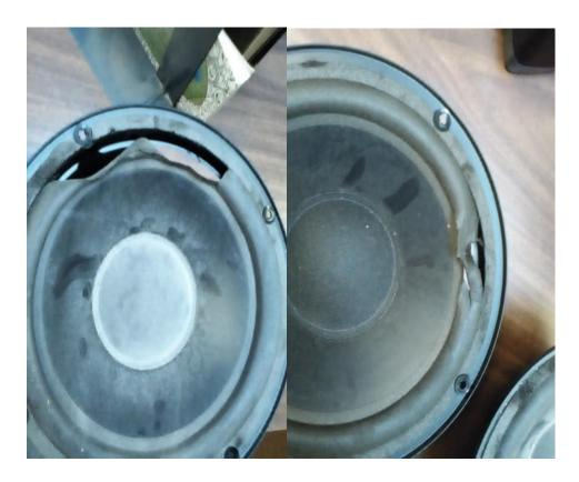
Pictured are two of the old speakers showing how the cones had separated from the mounting, causing major distortion. Also, lights in the music rack and on the pedalboard were updated to LED lighting.
